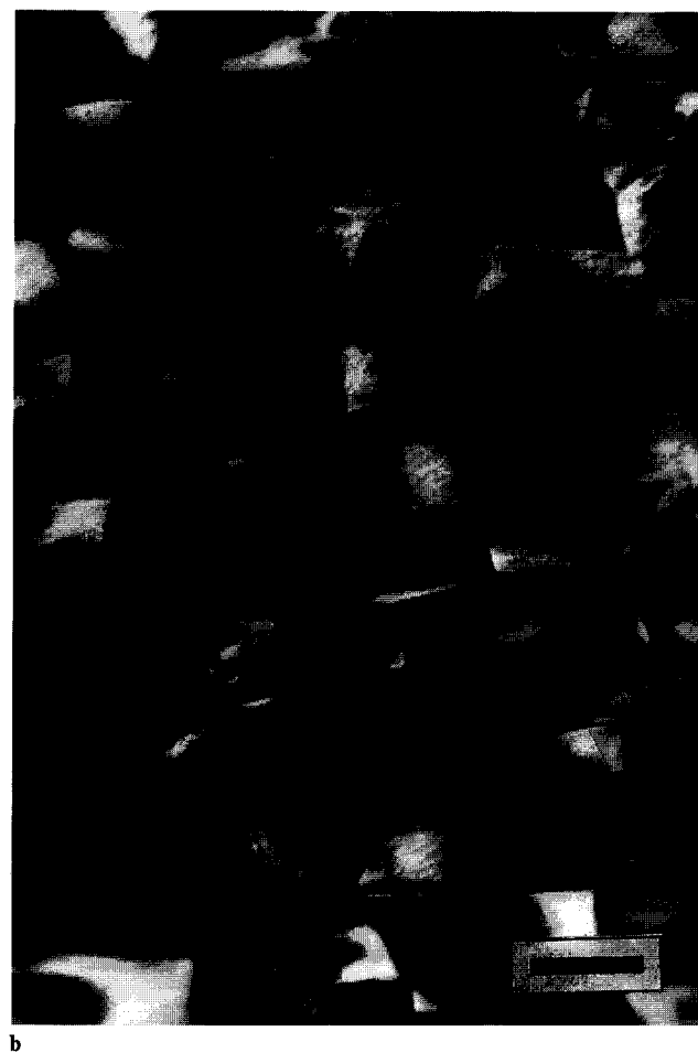
Figure 7 Micrographs of thin slices between crossed polarizers: (a) block copolymer (21.2% PA12); (b) PA6-PA12 blend (15.4% PA12); scale bar 20 μm
